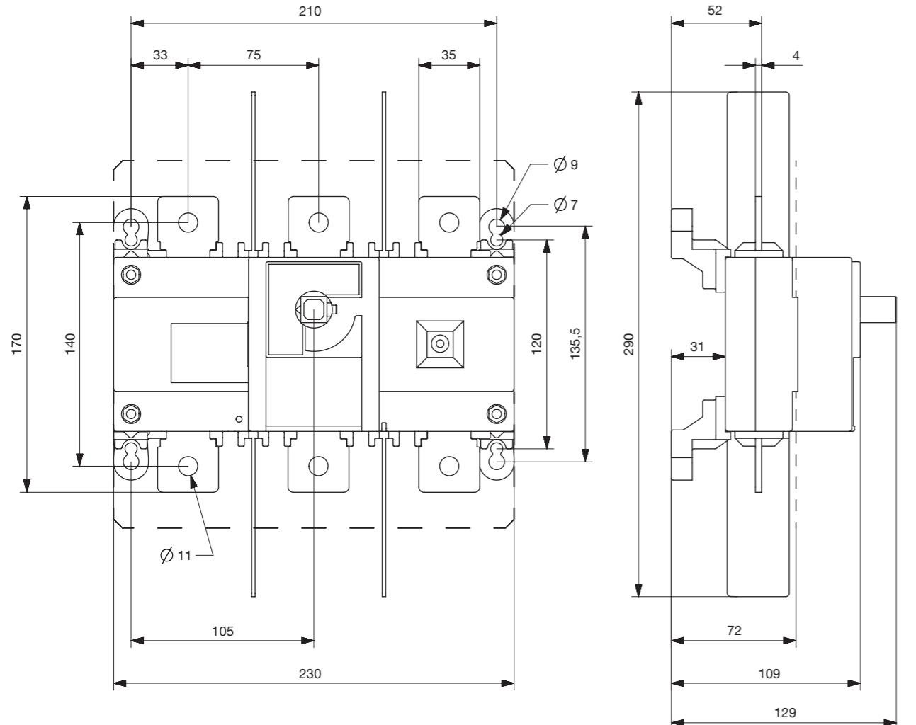
From 250 to 400 A - 1500 VDC: IEC 60947-3 [3 poles in series]
