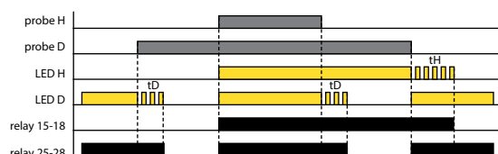
PUMP DOWN, OFF DELAY (Function 6)
